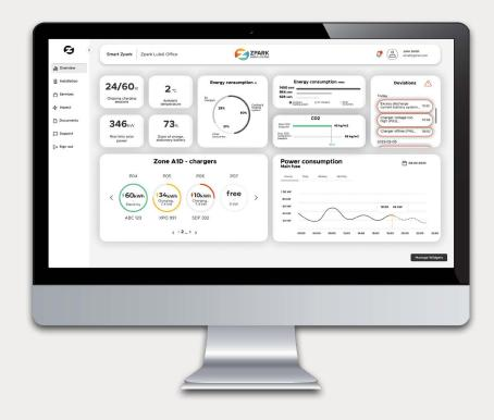
The Zpark Portal offers facility owners a comprehensive overview of the facility, with the ability to easily set the charger's mode as public, private, flexible, or always available. The portal also allows you to set pricing and cost schedules for both electric vehicle charging and engine heating. Through the portal, the facility owner gains complete control over the occupancy rate and access to detailed statistics for strategic planning and performance optimization of the parking spaces.
